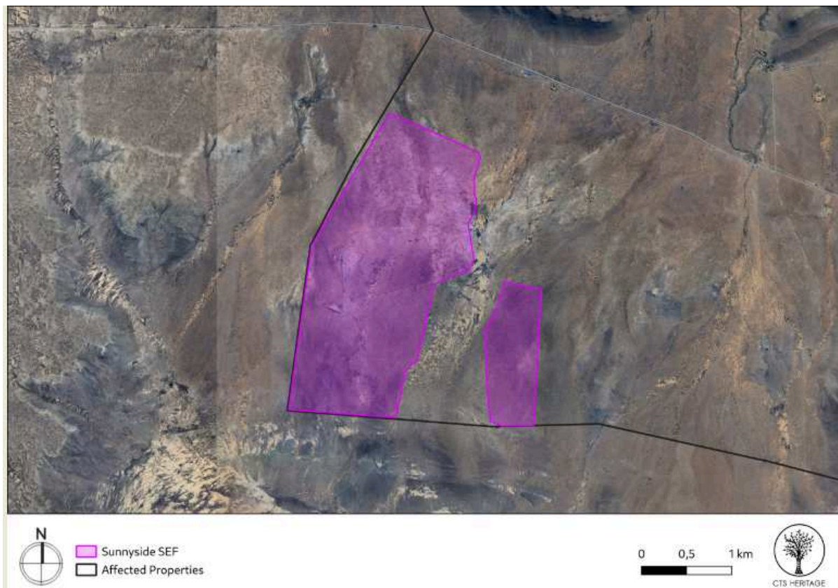
Figure 3: Google Earth© satellite image showing the Sunnyside SEF project areas (purple polygons) on Farm 400. The majority of the area is mantled by sandy to gravelly alluvial soils underlain by a calcrete-capped pediment surface. Bedrock exposure within the SEF project areas themselves is very low but occasional small patches of Beaufort Group mudrocks with diagenetic carbonate concretions occur further to the east (darker areas on satellite image).
