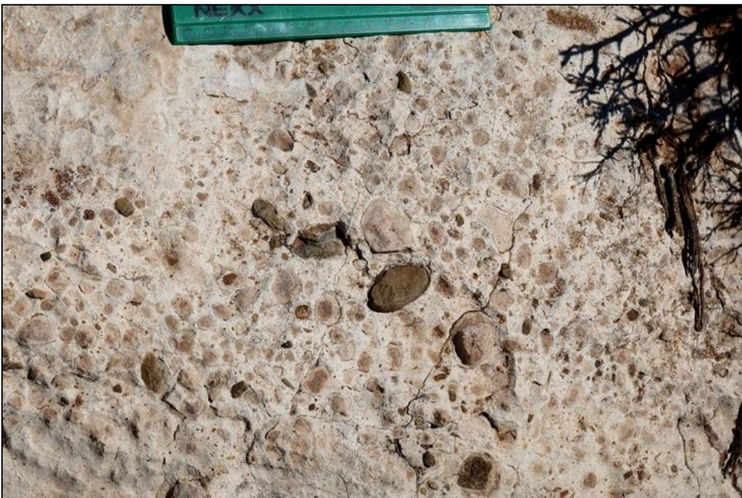
Figure 13: Close-up of the calcrete hardpan illustrated above showing composite nature with re-cemented, well-rounded and concentrically-laminated calcrete clasts (pisolitic texture) plus occasional gravels. Scale = c. 15 cm.
